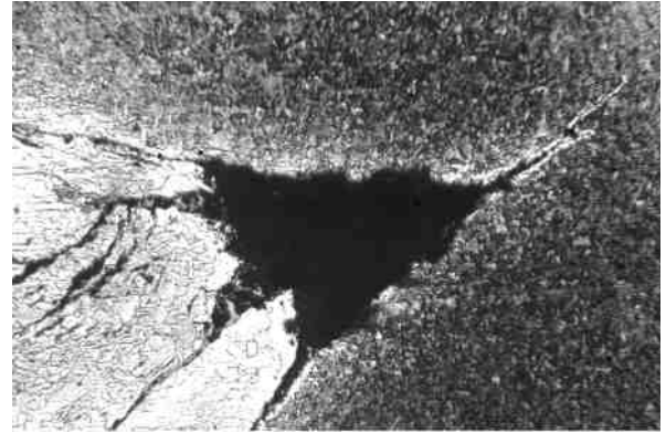
Fig. 55. An iron rivet in a hardened steel link from shirt RW2 (m1). Photo by A. Williams.
