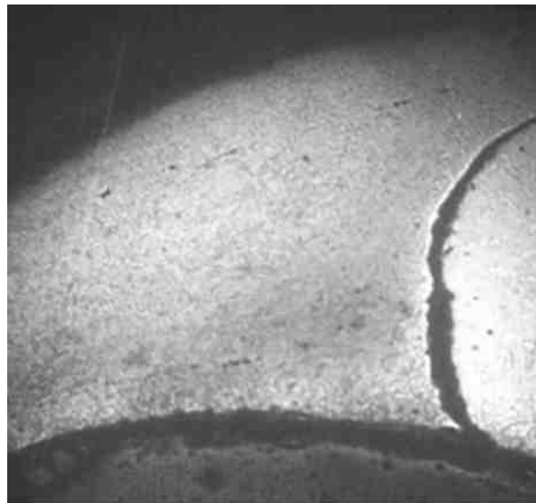
Fig. 62. A6 composite mail, ring 3 (body) – note the iron rivet in a hardened steel ring. Photo by A. Williams.
