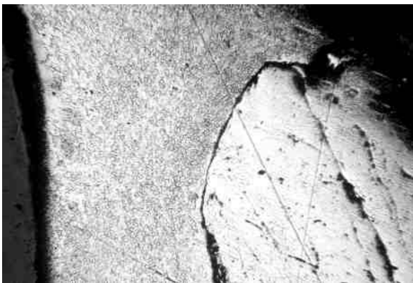
Fig. 47. An area around the rivet in the link from A3 (m2) (x 100). The rivet consists largely of iron, even though this would have been a weakness in the finished link. Photo by A. Williams.
