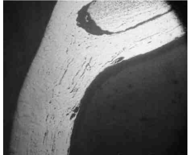
Fig. 66. A6 mail, ring 1 and rivet (seam) – ferrite and pearlite in the ring (part of the rivet is also visible). Photo by A. Williams.
