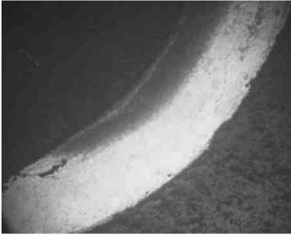
Fig. 63. A6 mail, ring 2 (patch) – Dark-etching martensite and a band of ferrite in the ring. Photo by A. Williams.
