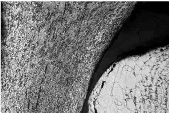
Fig. 44. An area around the rivet in the link from A2 mail (m1) (x 100). The rivet consists largely of iron. The grains in the link adjacent to the rivet show considerable distortion, cold to cold-working. Photo by A. Williams.
